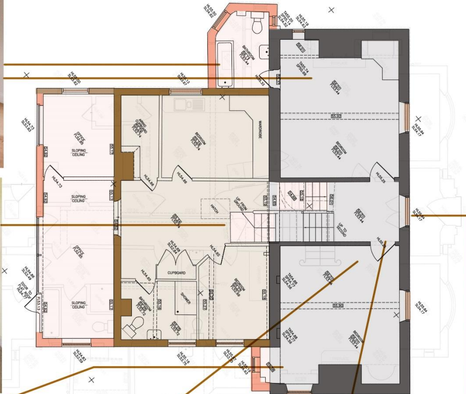
Stairs. Modern lower flight inserted under 18C winder.
