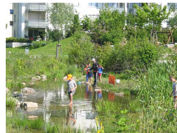
Shallow slopes, low water depth and stable edges minimise the need for fences and illustrate a design-led approach to health and safety
